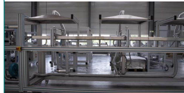
Drying/Curing via IR
