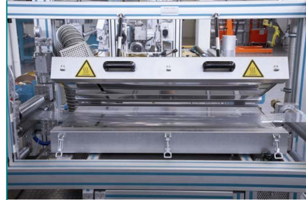
Drying via hot air
