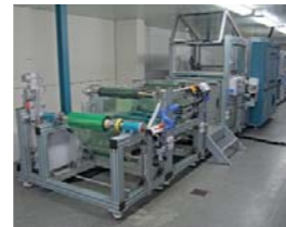
Click&Coat™ - Unit Working width: 500 mm
