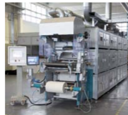
Linecoater Working width: 500 mm
