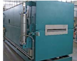
Inert drying system - Floation Dryer Working width: 500 mm
