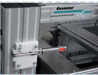
Click&Coat™: the individual plant components can be brought into the right position by a simple "click"
