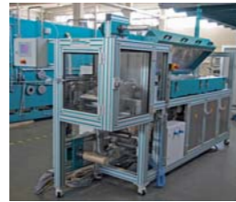
Basecoater Working width: 250 mm
