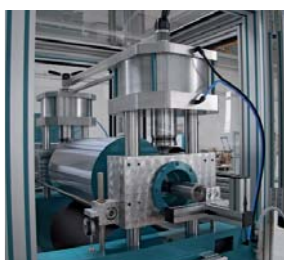
Click&Coat™: the individual plant components can be brought into the right position by a simple "click"
