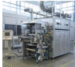
Deskcoater Working width: 500 mm
