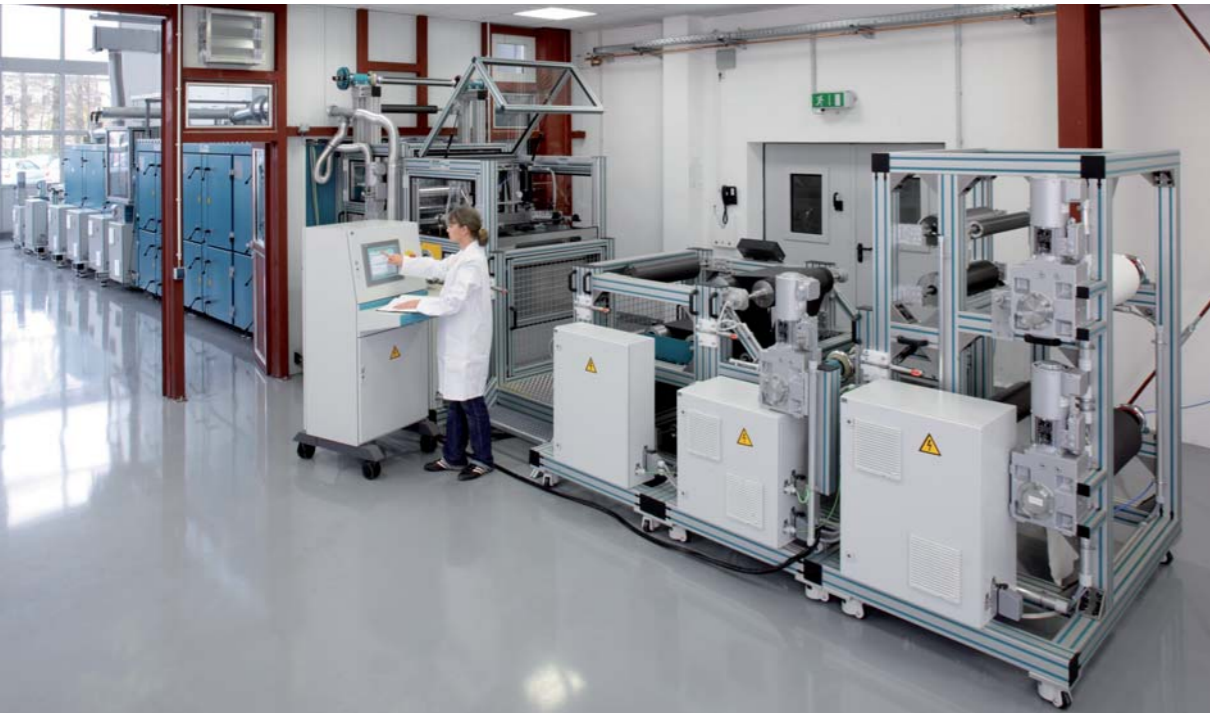
Click&Coat™ coating plant for the fuel cell production (Source: Forschungszentrum Jülich)
