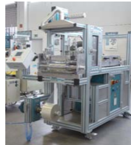
Basecoater Working width: 250 mm
