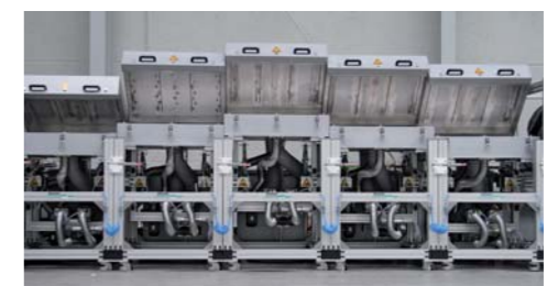
Click&Coat™: the individual plant components can be brought into the right position by a simple "click"
