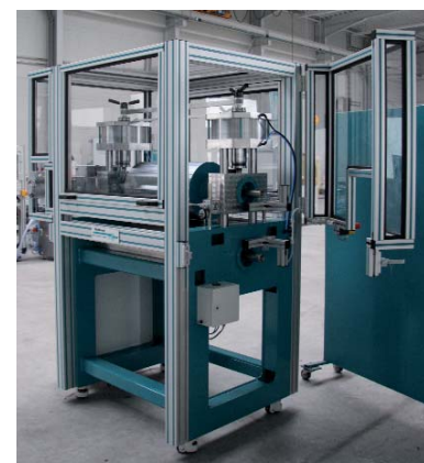
Calender with a load of 6 tons (pneumatic) Application area: Fuel Cell
