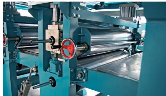
Calender with a load of 6 tons (pneumatic) and adjustable hot plates (pneumatic) Application area: Prepreg
