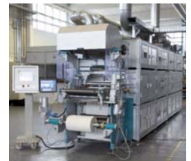
Linecoater Working width: 500 mm
