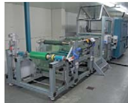
Click&Coat - Unit Working width: 500 mm
