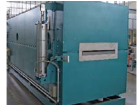
Inert drying system - Floatation Dryer Working width: 500 mm
