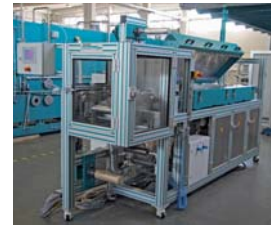
Basecoater Working width: 250 mm
