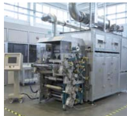
Deskcoater Working width: 500 mm
