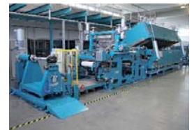
Multifunctional Coating Line Working width: 500 mm
