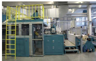
Unwinder, application system, laminating unit
