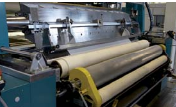
Application Systems: knife and roller coating system
