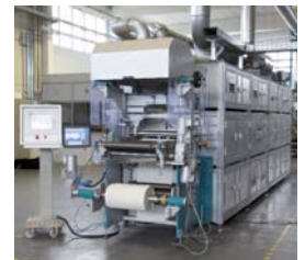
Linecoater Working width: 500 mm
