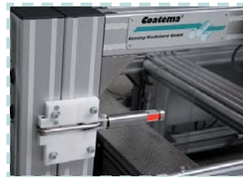
Click&Coat: the individual plant components can be brought into the right position by a simple "click"
