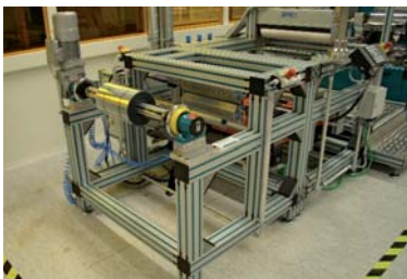
Unwinder and pre-conditioning
