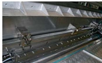
Slot Die application system
