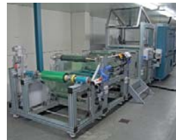
Click&Coat - Unit Working width: 500 mm
