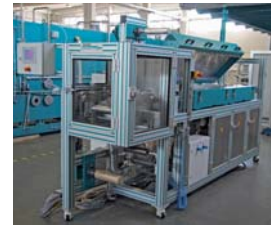
Basecoater Working width: 250 mm
