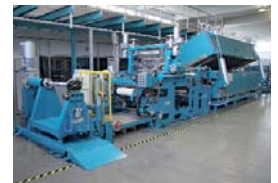
Multifunctional Coating Line Working width: 500 mm
