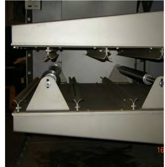
Nozzle dryers modul Dry with shifted nozzles and wing shaped blow boxes
