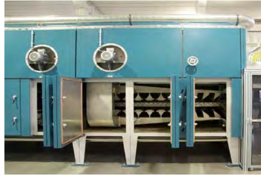
Wing shaped nozzle dryer with different nozzles
