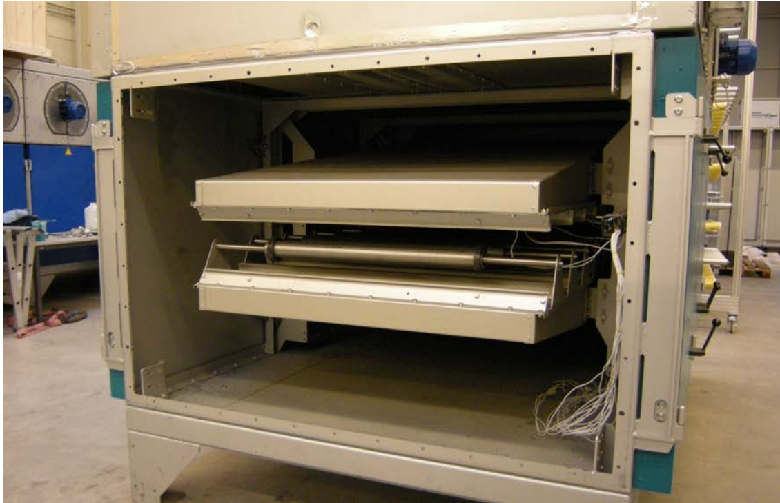
Nozzle dryers modul Dry with shifted nozzles and wing shaped blow boxes
