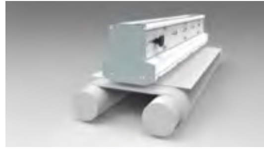
Flotation nozzles with adjustable air direction
