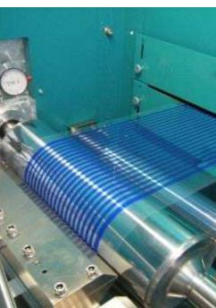
**Slot die coating** station compatible for materials used in OEs
